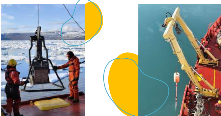
Box Corer (left) recovery after sampling the surface sediment in the Archer Fjord and Gravity Corer (right) ready to be deployed in the Conny Beare Fjord to collect longer sediment archives. Photos: J. Bonnín
